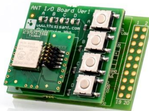
Figure 3-1. N5 Module stacked on IO and Battery Boards.
